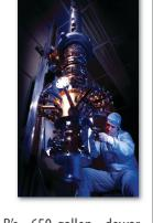
GP-B's 650-gallon dewar kept the science instrument inside the probe at a cryogenic temperature (2.3K) for 17.3 months and also provided the thruster propellant for precision attitude and translation control.
