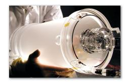
A telescope mounted along the central axis of the dewar and spacecraft provided the experiment's pointing reference to a "guide star." The telescope's image divider precisely split the star's beam into x-axis and y-axis components whose brightness could be compared.
